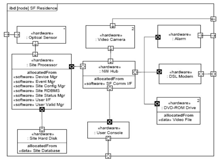
Used instead of deployment diagrams (artifacts allocated to nodes)
