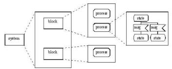
The leaf of the architecture is the process which is basically a finite state machine with an implicit message queue associated to it.
