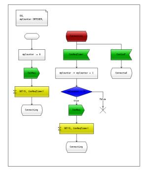
The example above shows a basic finite state machine: during initialization a *ConReq* message is sent out and a the *ConReqTimer* is started. The state machine goes to *Connecting* state and waits for the connection confirmation message *ConConf*, or the timer to go off. In the later case, the connection request is resent 10 times. If still unsuccessfull, the process is stopped.
